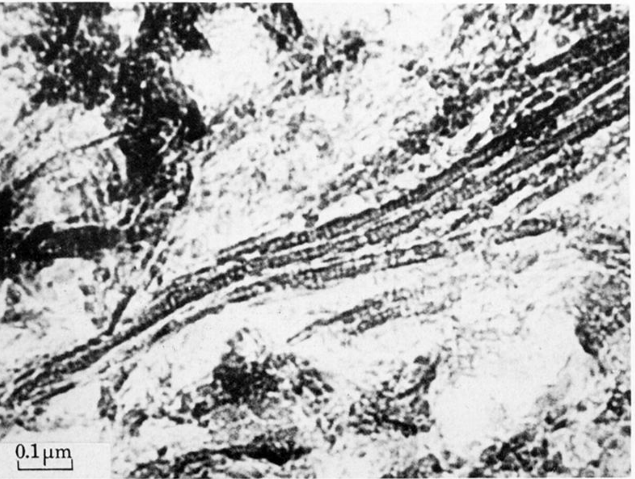
FIGURE 7. Lamellae of calcium hydroxide embedded in hydrate gel in a macro-defect-free cement paste.
